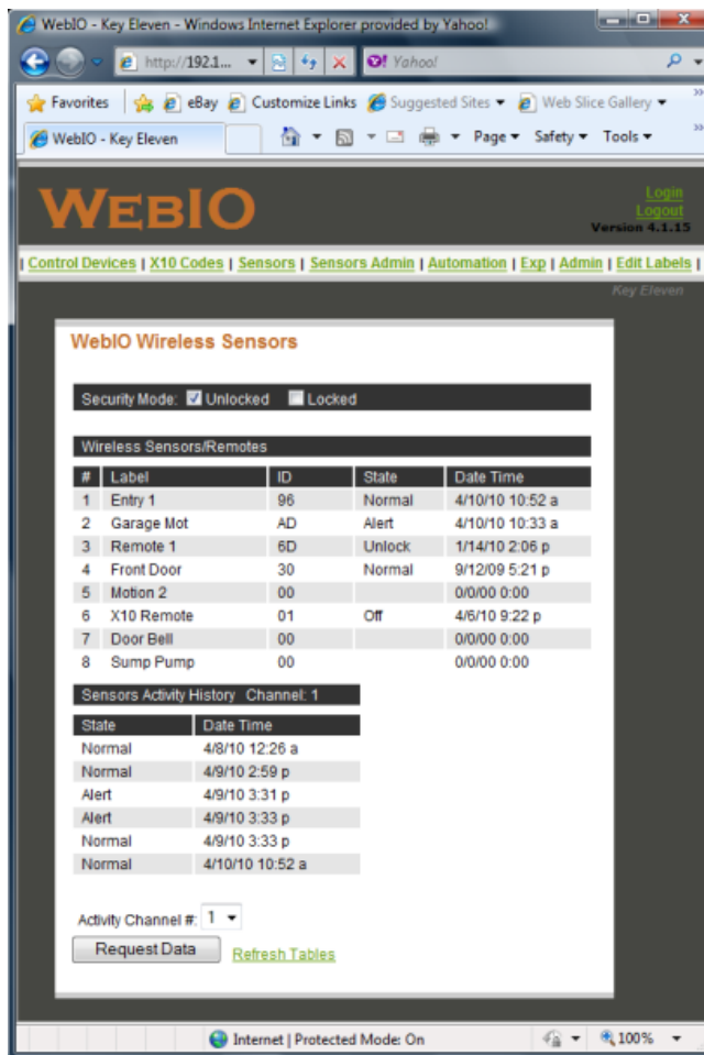
Figure 3: Connection to WebIO (Sensor page) using Internet Explorer web browser
